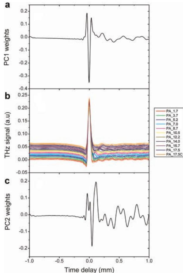
**Figure 4.** PLS loading-weights for PC1 (a), PC2 (c) and the terahertz waveforms (b) collected at 10% increments of the amount of coating polymer applied. PA is the amount of polymer applied in mg/cm<sup>2</sup>. C stands for cured tablets. The terahertz waveforms are offset for clarity.
