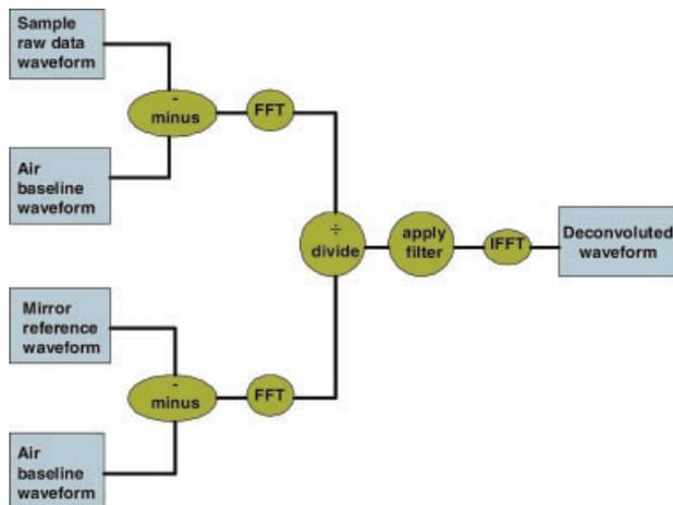
**Figure 2.** Terahertz time domain signal deconvolution. FFT stands for fast Fourier transformation and IFFT stands for inverse fast Fourier transformation.
