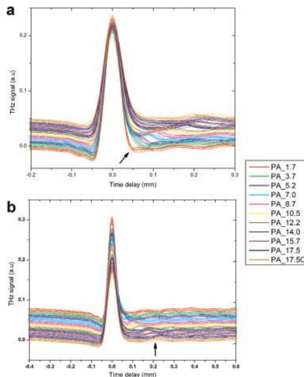
**Figure 6.** Terahertz waveforms of all samples from batch I. PA is the amount of polymer applied in mg/cm<sup>2</sup>. C stands for cured tablets. The changes in the postsurface reflection dip (at 0.04 mm time delay) are indicated by an arrow in (a). The shift in the interface reflection for tablets after curing is indicated by an arrow in (b). The terahertz waveforms are offset for clarity.
