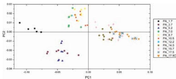
**Figure 5.** Scores plot of tablets sampled from batch I at 10% increments of the amount of coating polymer applied and from the finished product. PC1 and PC2 together explained 77% of the variation in the terahertz waveforms and 92% of the variation in the MDT data. PC1 traces the coating progress from the lowest polymer level on the left to the highest polymer level on the right; whilst PC2 mainly differentiates the 3.7 and 5.2 mg/cm<sup>2</sup> cluster from the rest of batch.
