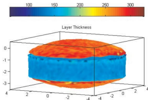
**Figure 1.** A 3D terahertz tablet scan of a round, biconvex tablet. The scales in the  $x$ ,  $y$  and  $z$  directions are in mm. The colour scale bar depicts layer thickness and the unit is in  $\mu\text{m}$ .
