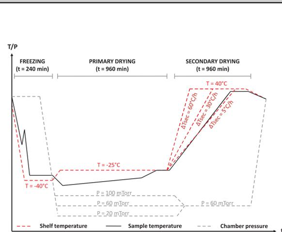
Figure 2. Primary drying chamber pressures ( $P_{prim}$ ) and secondary drying shelf ramping rates ( $T_{sec}$ ) used in the lyophilization experiments.
